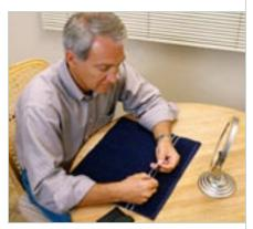
water. Be certain that the instrument is detached and far away from any moisture before cleaning. A brush may be provided to remove earwax or other particles that may have accumulated around switches and the battery compartment of your instrument. Never use solvents, cleaning fluids or oil to clean your instrument or earmold.
