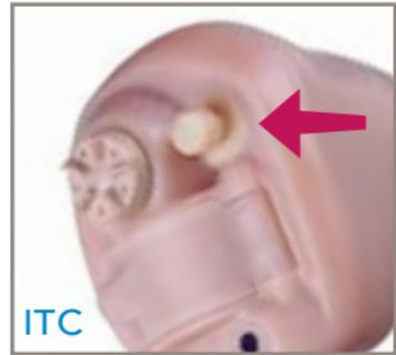
When turned on, your instrument is most likely programmed for normal listening environments. The additional settings are accessed by pressing the button once to select memory two and twice to access memory three.
