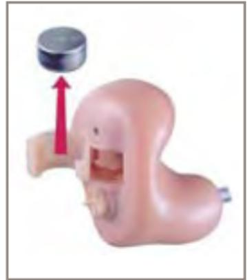
Existing batteries are removed by pushing the cell out the top of the fully opened door. **DO NOT** pull it out the side of the door.
