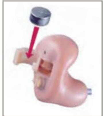
This could result in serious damage. If the door will not close securely, check that the battery is placed properly in the compartment.
