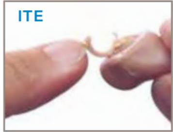
To insert or replace the battery, open the compartment by placing your fingernail under the edge of the swing-out door and gently pulling outward.
