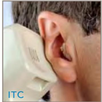
Effective telephone use with hearing instruments varies with the amplifier in your instrument. Those with either an automatic or manually switched telecoil enable you to comfortably use the tele-phone without removing your instrument. The induction coil amplifies the naturally emitted signal from the phone receiver.
