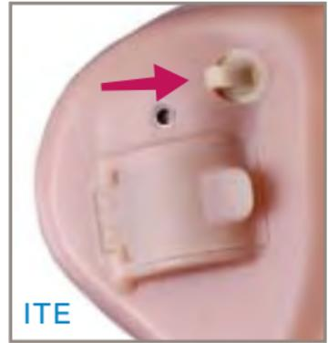
Instruments with the automatic telecoil will automatically activate when a properly equipped phone receiver is placed near the ear. Manually switched telecoils are activated by moving the switch to the "on" position.
