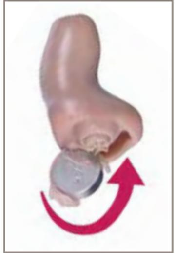
To turn the instrument "on," use your fingertip to rotate the volume control forward, toward your face. You should feel it "click" on if the instrument was correctly turned off. To make sounds louder, continue to rotate the control forward, toward your face.
