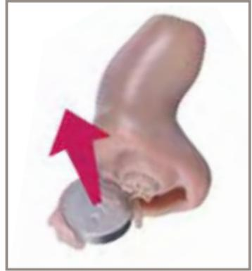
Existing batteries are removed by pushing the cell out the top of the fully opened door. **DO NOT** pull it out the side of the door.
