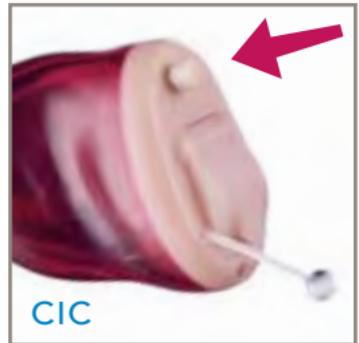
When turned on, your instrument is most likely programmed for normal listening environments. The additional settings are accessed by pressing the button once to select memory two and twice to access memory three.
