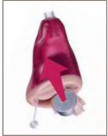
Existing batteries are removed by pushing the cell out the top of the fully opened door. **DO NOT** pull it out the side of the door.
