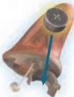
Close the battery compartment by swinging the door until it snaps securely. **NEVER FORCE THE DOOR SHUT.** This could result in serious damage. If the door will not close securely, check that the battery is placed properly in the compartment.
