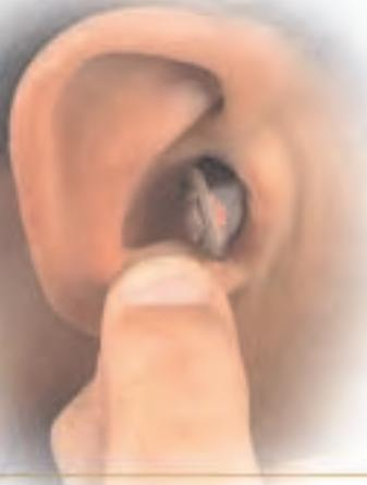
Let go of the insertion/removal line, and push the instrument in until it is resting comfortably inside your canal. To ease insertion, you may wish to pull down on your ear lobe with your other hand as you push.
