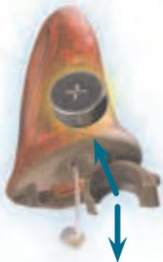
Remove the existing battery either by pushing it out the bottom of the door, or pulling it straight out.
