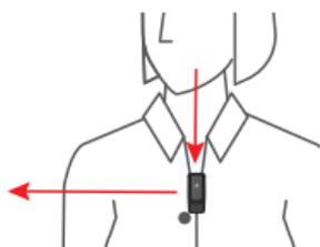
**"Surround"** – When SurfLink Remote Microphone is placed horizontally (on its clip), it receives sound from all directions. This setting is useful for listening to multiple nearby speakers in quiet environments.
