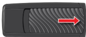
2. Press "Sync" icon on slider button for 5 seconds until LED starts rapidly blinking blue.
