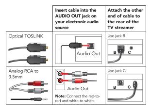
**Tip:** During initial setup, a solid blue LED confirms the audio cable is properly attached to the TV streamer and audio streaming is active.
